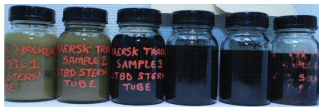
6 oil samples from the Total Disola M 4015 oil - taken over a 4-week period.
