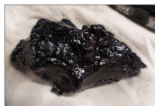
Asphaltenes due to residues of heavy fuel in the tank.
