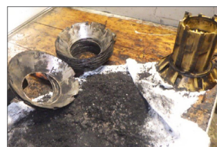
Asphaltenes on components from the centrifugal purifier.
